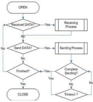
Fig 15. IPRAW Operation Flow
