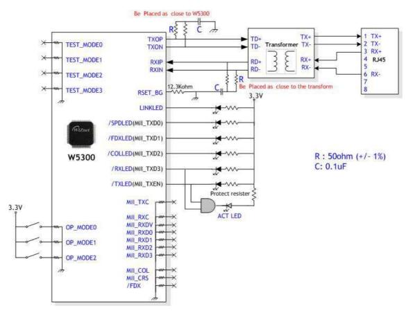
Fig 19. Internal PHY & LED Signals
