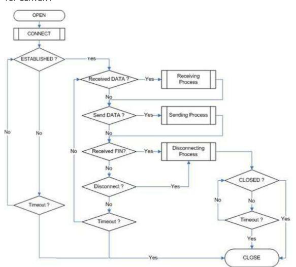
Fig 12. "TCP CLIENT" Operation Flow
