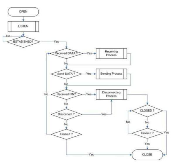
Fig 10. "TCP SERVER" Operation Flow
