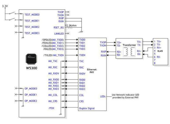
W5300's '/FDX' Pin is connected to duplex indicator signal of the external PHY.
