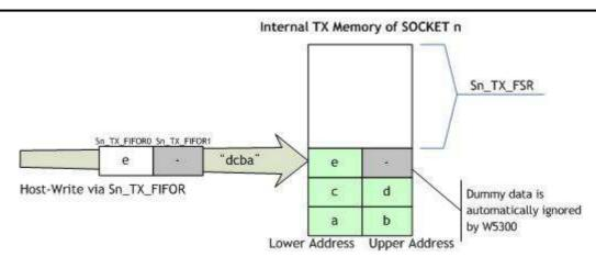
Fig 6. Access to Internal TX Memory
