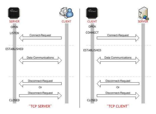
Fig 9. "TCP SERVER" & "TCP CLIENT"
