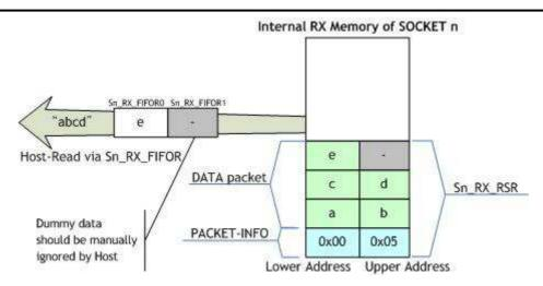
Fig 7. Access to Internal RX Memory
