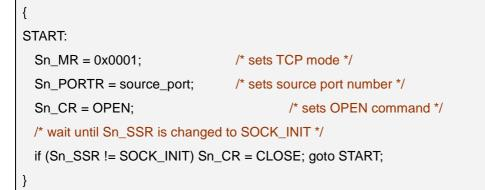
If all data size received from the peer are even number,  $Sn_MR(ALIGN)$  can be set as '1'. In case of  $Sn_MR(ALIGN) = '1'$ , W5300 does not add the PACKET-INFO of TCP mode, and save only DATA packet in internal RX memory of SOCKETn. This can improve the performance by reducing the host's overhead of PACKET-INFO process. (In above code,  $Sn_MR = 0x0101$  can be replaced with  $Sn_MR = 0x0001$ )
