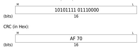
Putting it together (PID + 18 bytes of data + CRC):
