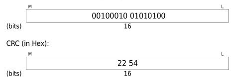
Putting it together (PID + 13 bytes of data + CRC):
