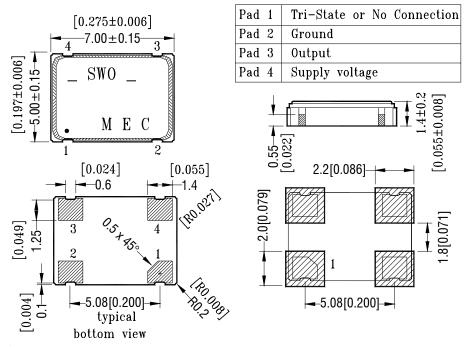
Chamfered paad is pad No. 1. Count counter-clockwise when looking at top view. Count clockwise when looking at bottom view.
