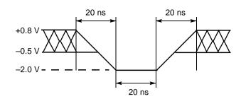
Figure 5. Maximum Negative **Overshoot Waveform**
