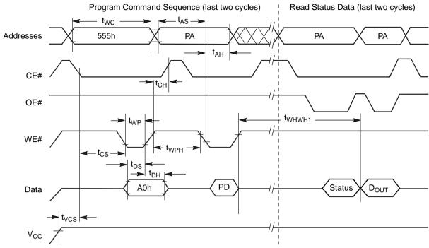
**Note:**  $PA = program \ address, PD = program \ data, D_{OUT}$  is the true data at the program address.
