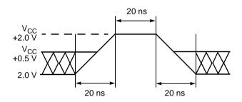
Figure 6. Maximum Positive Overshoot Waveform
