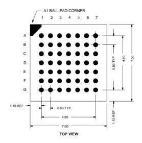
Figure 2: Pin Configuration, BGA-49.
