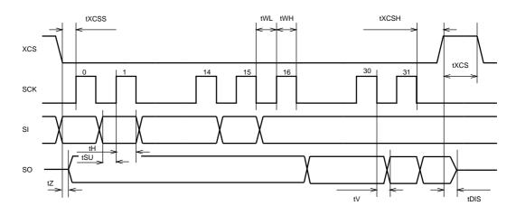
Figure 8: SPI Timing Diagram.
