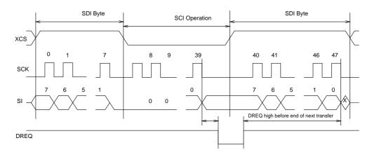
Figure 11: Two SDI Bytes Separated By an SCI Operation.
