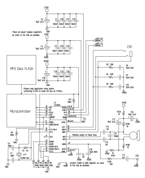
Figure 3: Typical Connection Diagram Using LQFP-48.
