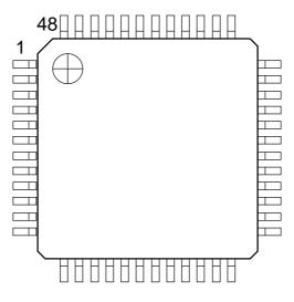
Figure 1: Pin Configuration, LQFP-48.
