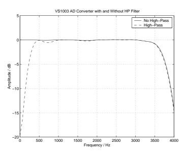
Figure 13: ADPCM Frequency Responses with 8kHz sample rate.
